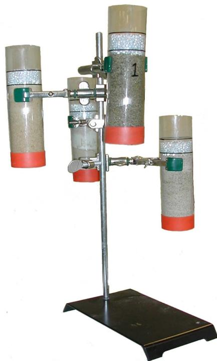
Ringstand set-up for Flow-through activity (one per group)
